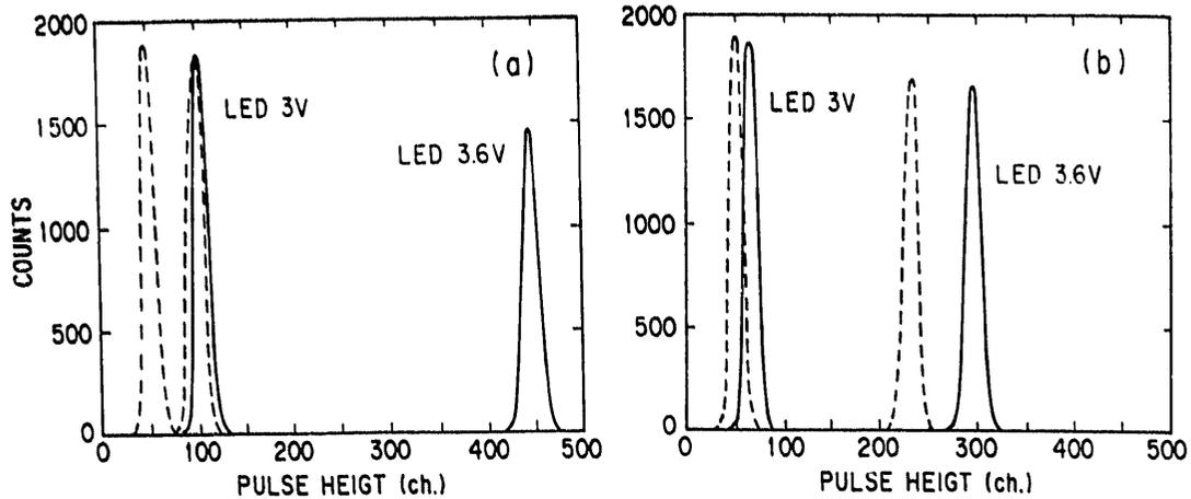
Fig. 3. Typical distributions of the output signal. (a) Signal from R239 (bialkali) at 0°C (solid line) and -110°C (dotted line). (b) Signal from R1221 (multialkali) at 0°C (solid line) and -180°C (dotted line). The LED is operated at 3 and 3.6 V.
