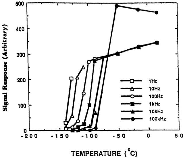
Fig. 6. The signal response versus temperature for a R329 photomultiplier. The luminous intensity dependence is seen.
