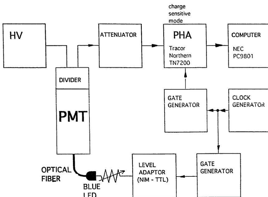
Fig. 2. The block diagram of the data-taking system.
