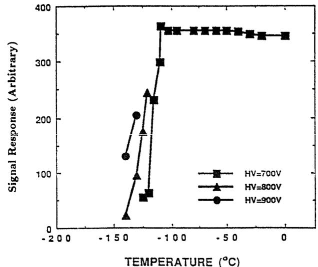
Fig. 5. The high tension dependence of the bialkali R464 photomultiplier.
