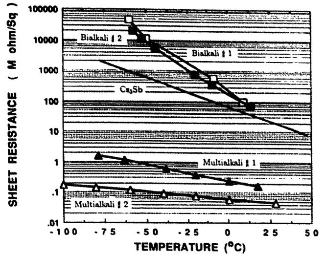
Fig. 8. The sheet resistance of different photocathodes as function of temperature.
