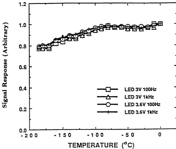
Fig. 7. The signal response vs temperature for a R1221 photomultiplier.
