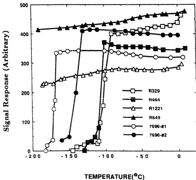
Fig. 4. The temperature dependence of the output pulse for different types of photomultipliers.
