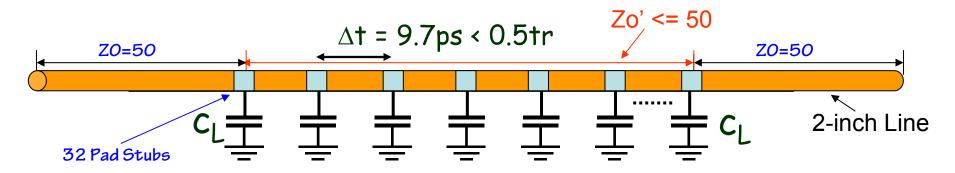
Equal distributed 32  $C_L$ =100f along 2-inch line, It reduces impedance to Zo', However, it also reduced the BW.
