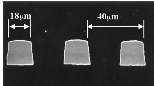
Fig. 4. 40  $\mu\text{m}$  pitch circuitization on 1-metal layer FLEX (see text).
