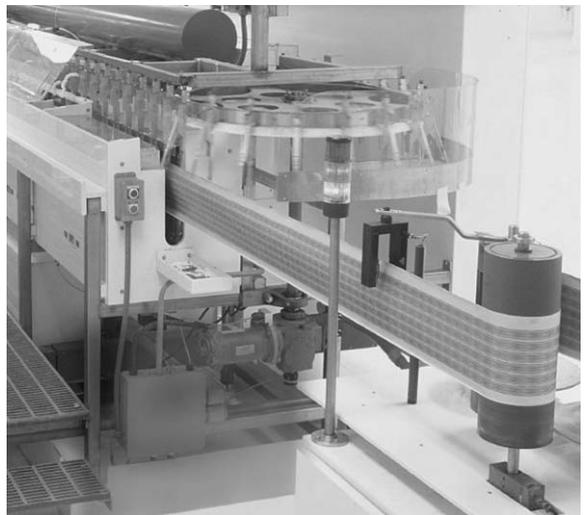
Fig. 2. 3M's roll-to-roll flexible circuit manufacture in clean room conditions.
