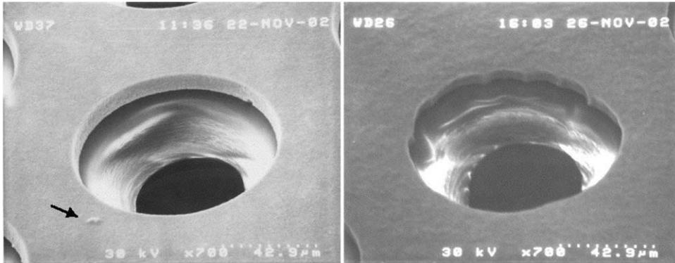
Fig. 5. Scanning electron microscope images of 3M subtractive (left) and additive GEMs (right). A small Cu microcrystal (height  $< 1 \mu\text{m}$ ) is indicated by an arrow on the subtractive surface. No sparking or other spurious effects have been observed from these. Additive GEMs display smoother surfaces but copper opening irregularities can be identified on large areas of the panels. An extreme case is depicted here (see text).
