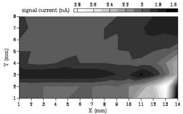
Fig. 9. Gain uniformity in Ar:DME (9:1) for a subtractive 3M GEM irradiated with a strong  $5.4\text{ keV}$  X-ray source focused on a  $1\text{ mm}^2$  spot. The current generated was measured with a picoammeter directly from the bottom GEM electrode ( $V_{\text{drift}} = 600\text{ V}$ ,  $V_{\text{GEM}} = 400\text{ V}$ ). The measured dispersion (standard deviation of 112 measurements) is 9%.
