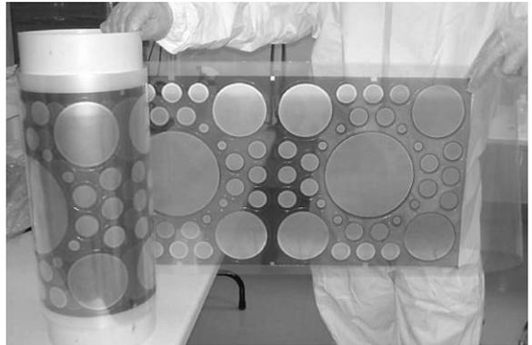
Fig. 1. Single continuous roll containing a production of  $\sim 1000$  subtractive GEM elements in different sizes. Barely visible in the figure are perforations made around each GEM to facilitate detachment. The maximum GEM area permitted at present in 3M's production line is  $30 \times 30 \text{ cm}^2$ , already comparable to the largest MPGDs produced for high-energy physics experiments.
