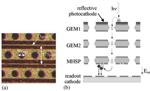
Fig. 7. A photograph of the striped side of an MHSP electron multiplier (a) and a schematic layout of a gaseous photo-multiplier comprising a cascaded 2-GEM plus MHSP electron multiplier (b); signals are induced on a segmented cathode, providing photon localization.
