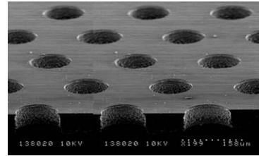
Fig. 8. A photograph of a perforated silicon substrate, studied for future GEM production. Si thickness: 120  $\mu\text{m}$ ; hole diameter: 100  $\mu\text{m}$ ; spacing: 200  $\mu\text{m}$ .
