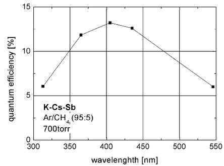
Fig. 6. The absolute quantum efficiency as function of wavelength of a visible-sensitive multi-GEM photomultiplier, sealed in atmospheric Ar/CH<sub>4</sub> (95/5).
