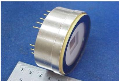
Fig. 5. A photograph of a sealed multi-GEM gaseous photomultiplier.
