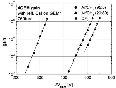
Fig. 2. Gain curves recorded in a multi-GEM photomultiplier with a reflective CsI photocathode, shown in Fig. 1b.  $\Delta V_{\text{GEM}}$  is the voltage across a single GEM.
