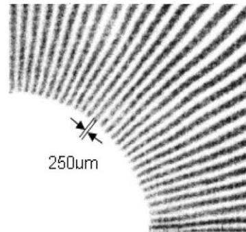
Fig. 4. A 2D X-ray image of a patterned mask of a total size of  $18 \times 18 \text{ mm}^2$ , recorded in a 3-GEM detector with a striped anode and delay-line readout; Ar/CO<sub>2</sub> (70/30), 1 atm.
