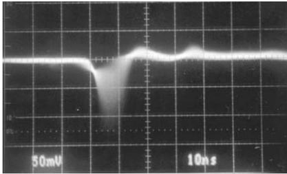
Fig. 3. Typical single-photon fast current pulses recorded in CF4 at a gain of 105.
