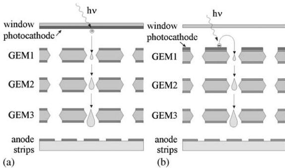
Fig. 1. Schematic view of the multi-GEM gaseous photomultiplier with: (a) a semitransparent photocathode and (b) a reflective photocathode. Signals are recorded at a segmented anode used for photon localization.
