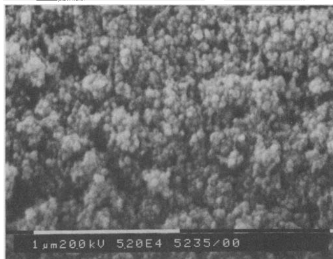
Fig. 8. Scanning electron microscope photographs of the Al 2 O 3 film deposited 200 cycles at 700°C.
