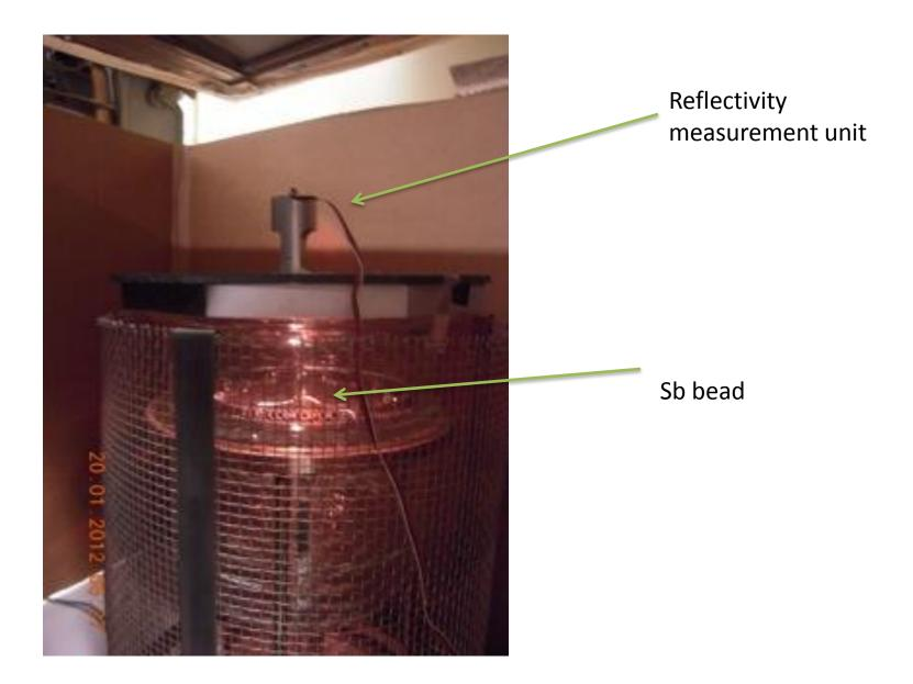
After overnight baking Note: the right down corner Sb blew out area, thin films can also be identified around the clear area.
