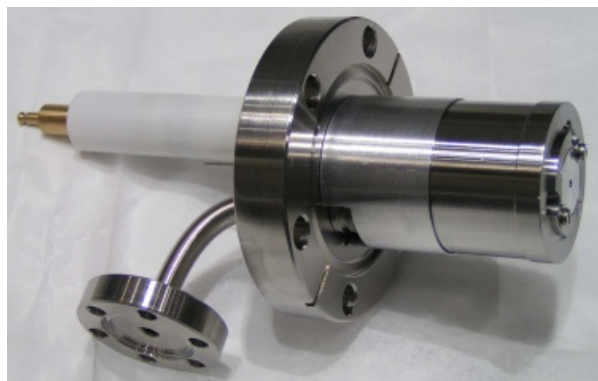
Figure 4.24: Saddle field ion gun detail, showing beam exit
