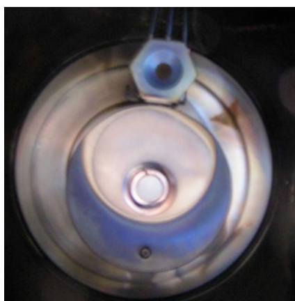
Figure 4.23: Deposition monitor above anode-cathode assembly inside vacuum chamber
