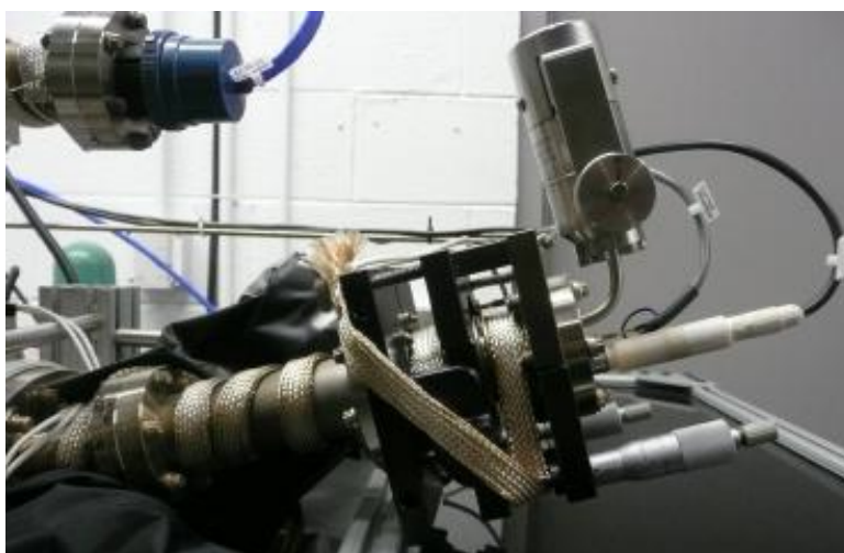
Figure 4.25: Ion gun and adjustable mount with argon fine leak valve
