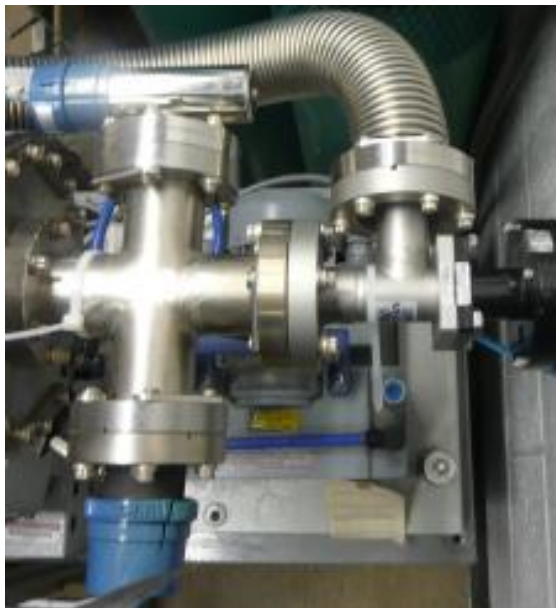
Figure 4.3: Turbopump manifold with pressure gauges and electromechanical valve
