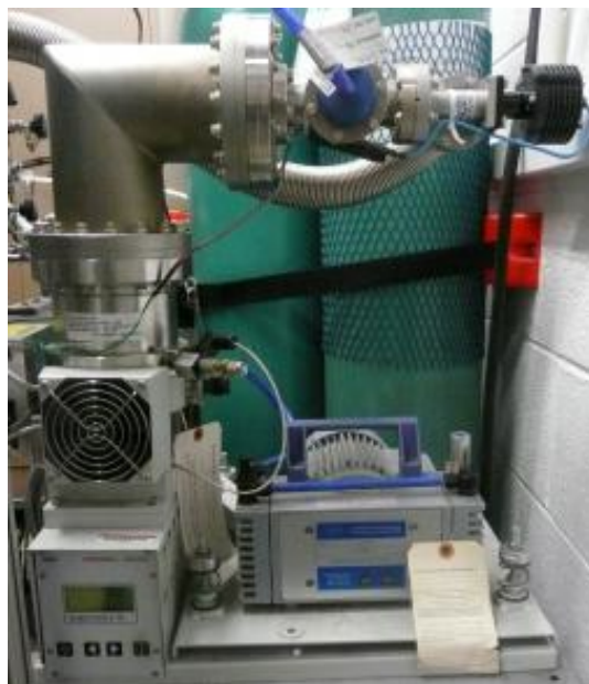
Figure 4.2: Turbopump station with scroll roughing pump
