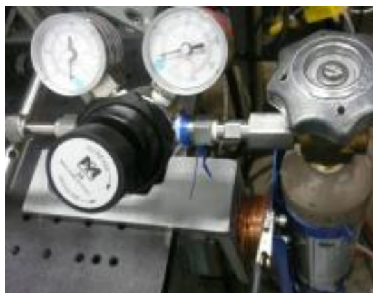
Figure 4.18: Detail of miniature regulator and interchangeable lab bottle
