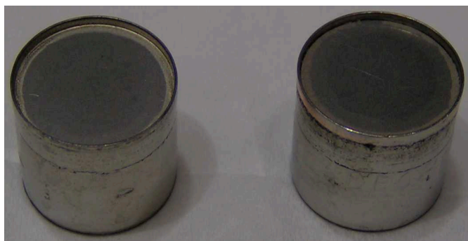
Figure 4.28: New dispenser, left, versus used dispenser, right, showing faint copper sputtering on outer top rim edge
