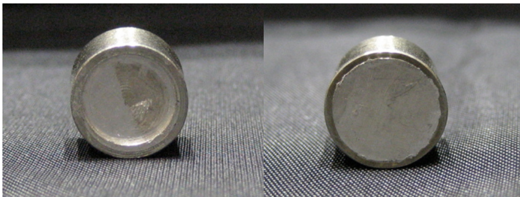
Figure 9.5: Custom Cs:Bi reservoir cartridge from Alvatec: (left) indium seal, (right) rear seal
