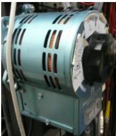
Figure 4.10: Variac (variable AC transformer) for cathode heater power control
