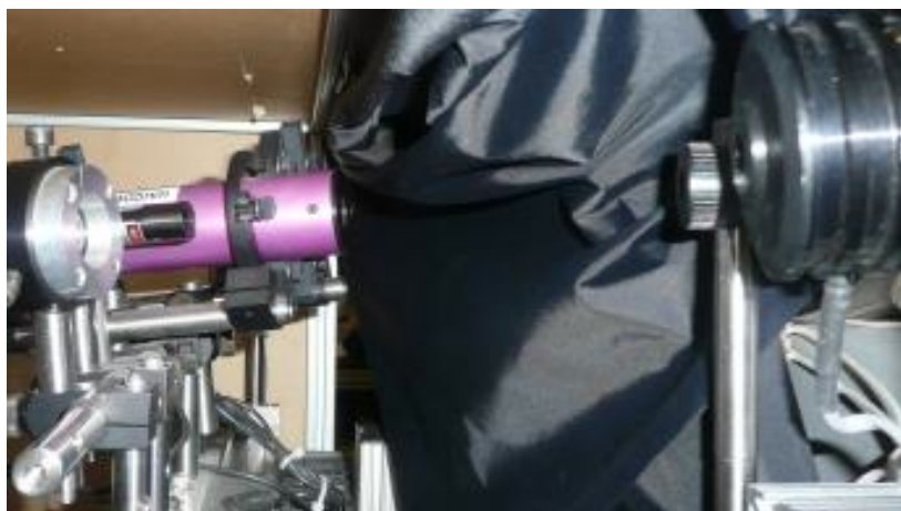
Figure 4.6: Lasers on translational mounts with thermopile power meter for auto-calibration
