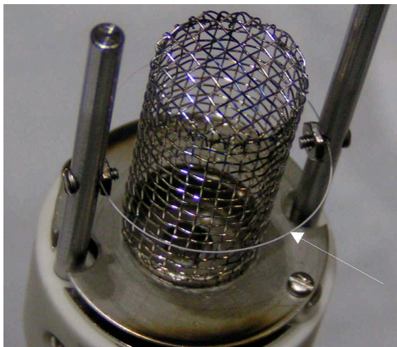
Figure 5.1: RGA filament, thoriated tungsten
