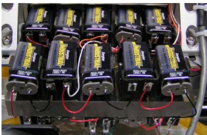
Figure 4.9: Isolated low-noise anode-cathode voltage supply
