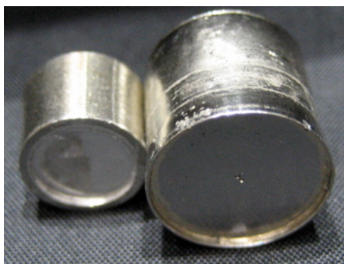
Figure 9.5: Custom Cs:Bi reservoir cartridge from Alvatec: (left) indium seal, (right) rear seal
