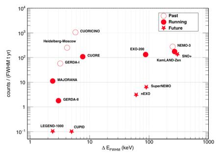
The background index as a function of full-width-at-half-maximum energy resolution for selected past, current and future experiments with 76Ge, 100Mo, 130Te, and 136Xe as target. Note that large homogeneous detectors like SNO+, KamLAND-Zen, and nEXO are not well characterized by a single background index.
