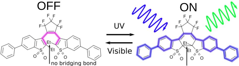
Highly transparent to visible light Can absorb a UV photon and turn ON by changing shape and electronic structure bridging bond causes extended fluorescent orbital
