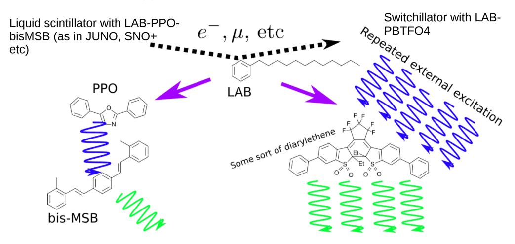
In a scintillator, the fluorescent dyes fluoresce and give you <1 photon to detect; JUNO targets >1200 photoelectons/MeV out of ~9500 photons/MeV
