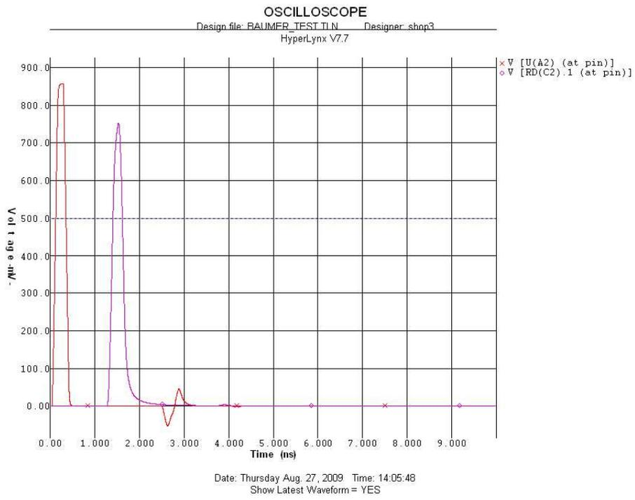
This is the response of the line with a 1mm thick kovar wall.
