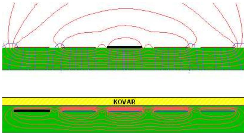
This figure compares the normal anode field geometry with the new geometry induced by kovar walls. The density of red potential lines indicates the strength of the coupling.
