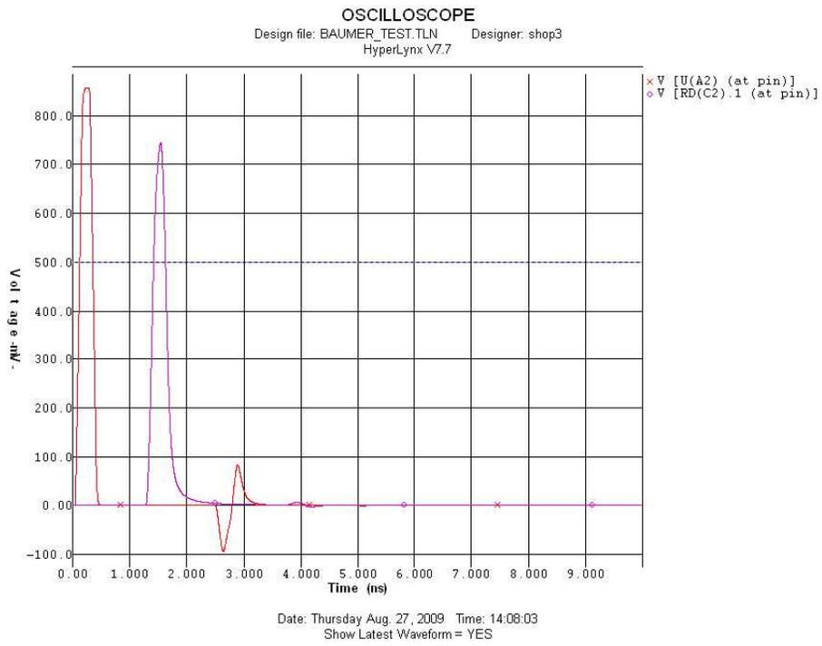
This is the response with a 2mm thick kovar wall.
