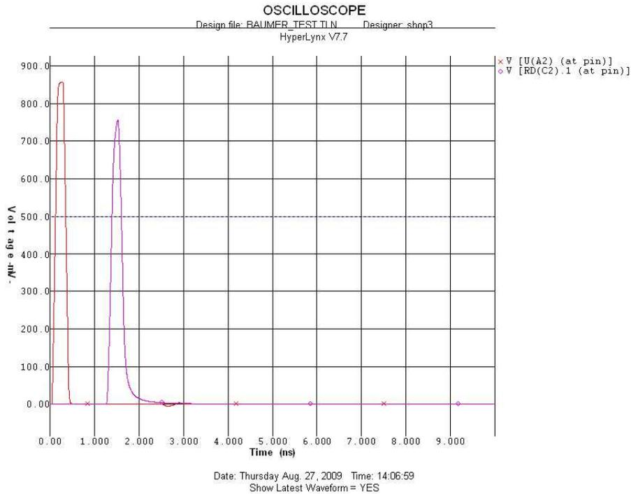
This is the response of the anode card by itself on a matched terminating resistor. Red is the input ( $\tau \approx 100ps$ ) and purple is the output.
