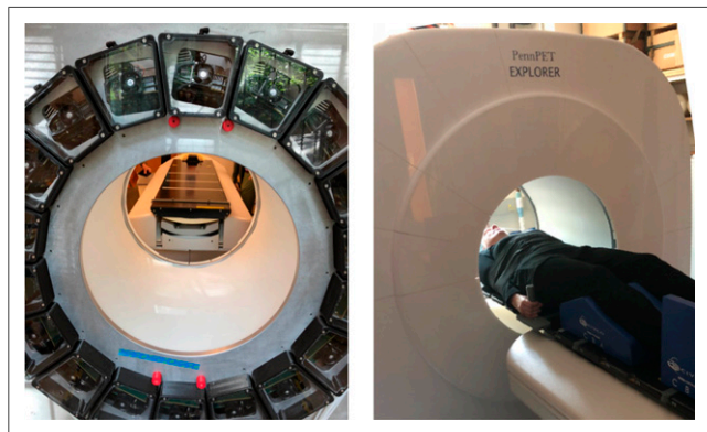
FIGURE 1. PennPET Explorer in its prototype configuration with 3 ring segments, housed in dry, cool enclosure. View of back of gantry shows modular detector and electronic bays. Also shown is couch with flat pallet installed for human studies.
