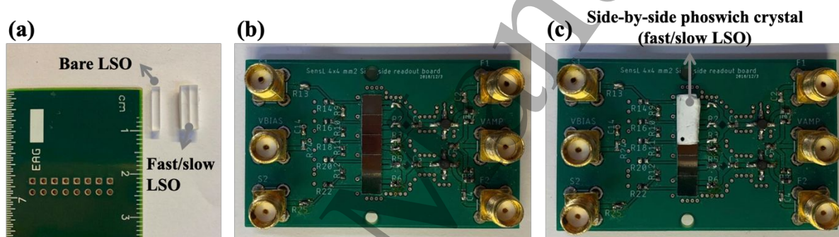
Figure 4 (a) Bare 1.9 \times 1.9 \times 10 \text{ mm}^3 LSO scintillator crystal (left) and phoswich arrangement with fast and slow LSO crystals (right) wrapped with Teflon tape. (b) 5 \times 1 array of 4 \times 4 \text{ mm}^2 SiPMs (c) Proposed side-coupled phoswich detector design arrangement. The black dot in the scintillator pair indicates where the fast crystal was positioned.
