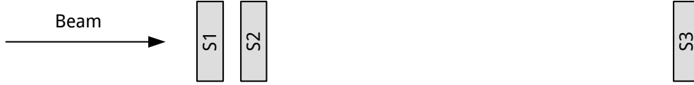
Figure 1: The scintillator telescope setup used for the measurement of the muon beam profile and intensity.
