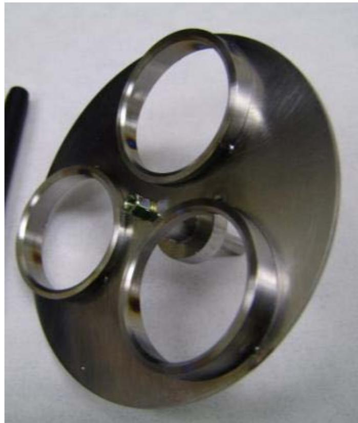
Fixture is shown loaded with one Incom glass plate in lower opening. When rotation angle of plate is properly aligned, the text below is clear. Otherwise, it is blurry. Red dot marks the inclination direction of the 8° bias angle pores. This demonstrates that the fixture holds the plates at the appropriate orientation for controlling the end spoiling during evaporation.
