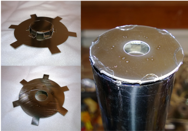
Fig. 2. (Color online) Details of the insets used to avoid direct line of sight between the azides in the crucibles and the substrate where growth is occurring.
