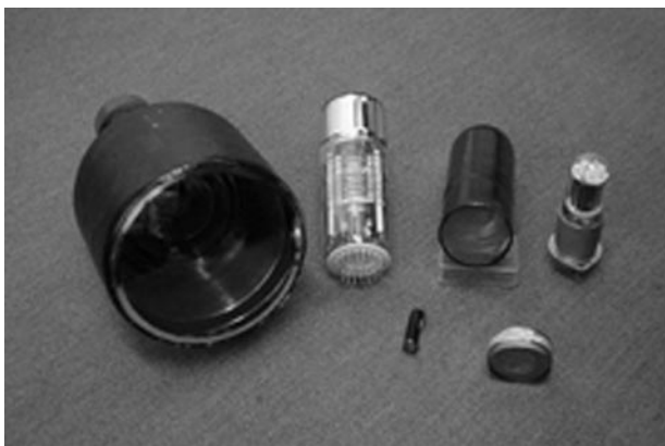
Figure 2. Some examples of photomultiplier tubes and an image intensifier. Larger or different shape tubes also exist. Ability to see into the tubes emphasizes the lack of cathode absorption.
