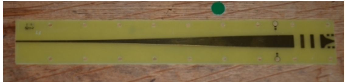
microwave taper 50 \rightarrow 150 Ohm to triple pulse amplitude 70V \rightarrow 210V
