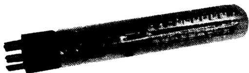
Fig. 2 - Magnetic-type multistage photomultiplier reported by Zworykin, Morton, and Malter in 1936.
