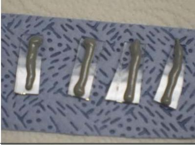
DT430 frit after drying. Note some spreading and leveling of the applied frit. At this stage the frit is not glazed. It remains friable and is easily wiped from the glass surface.
