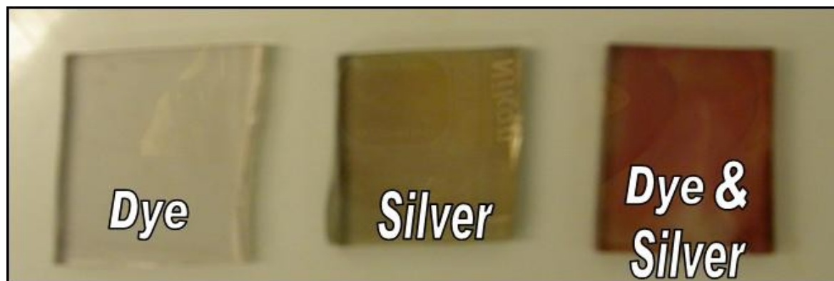
Fig. 16. a) N719 dye on low-area (flat) \text{TiO}_2 electrode, b) silver nanoparticle-coated, low-area (flat) \text{TiO}_2 electrode, c) N719 dye on \text{TiO}_2 (ALD)-coated silver nanoparticle layer on electrode. Quantitative measurements indicated ca. 5 to 7 fold enhancement in dye absorption in the presence of silver particles.
